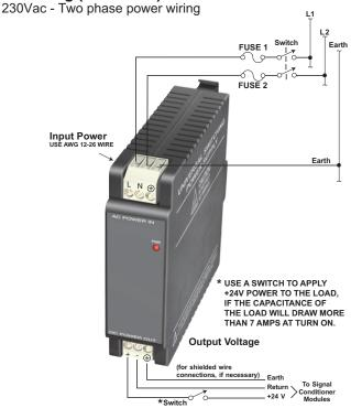
Figure 4.3— Wiring for 230Vac - Two Phase
